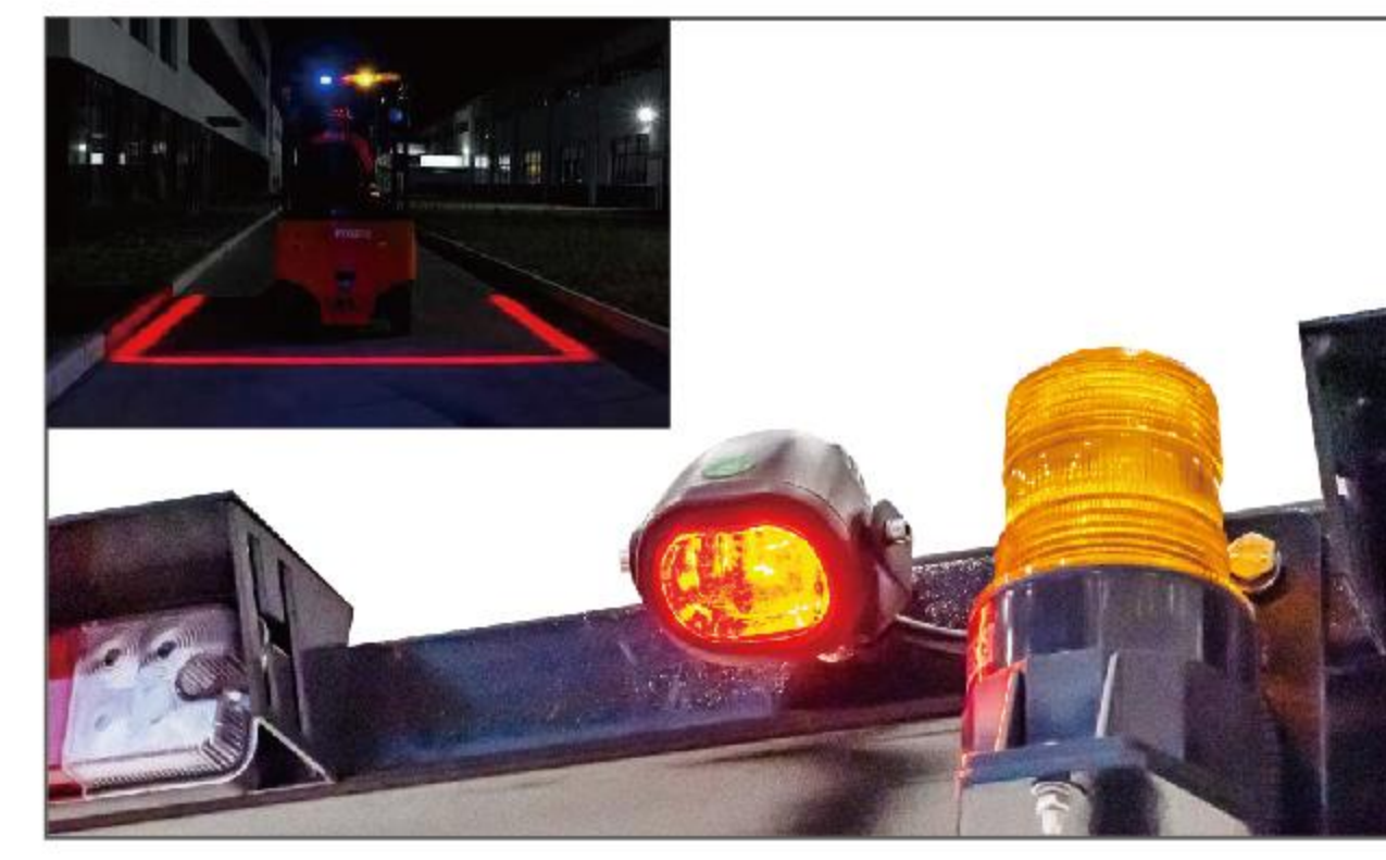
Red Safety Area Lights
